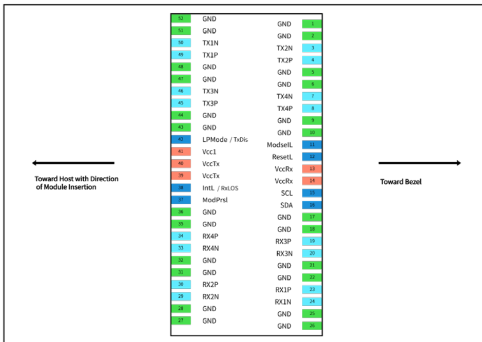
Figure 3 QSFP112 Host PCB pad assignment
